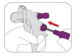
Reassemble in the following order: the needle spring and then the fluid adj. knob set.
