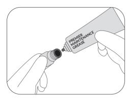
**9** Lubricate the fluid needle ajd. knob with a small amount of maintenance grease.
