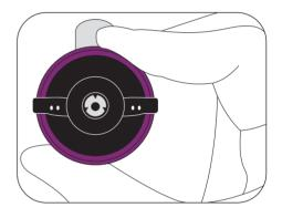
4 Once reassembled, align the air cap horizontally and tighten it by hand.
