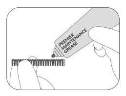
8 Lubricate the fluid needle spring with a small amount of maintenance grease.
