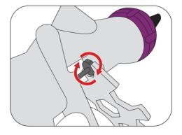
Now attend to the adjustment of the fluid needle packing. Screw the needle packing nut tight by the spanner until the needle starts to stick.
