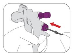
7 Insert the lubricated fluid needle set carefully into its seat.
