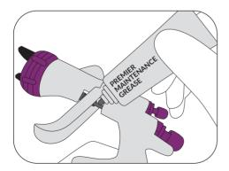
**11** Apply a small amount of grease to the fluid needle in the trigger slide area.
