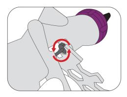
Once the needle sticks, unscrew the needle packing (counter-clockwise) until the needle just moves freely again.
