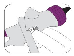
Place the self-adjusting needle packing in its seat and tighten it manually.
