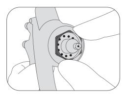
1 Reassemble the fluid nozzle tightening it manually into its seat.
