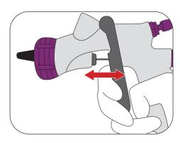
14 Check the smooth sliding of the fluid needle by pulling the trigger few times.
