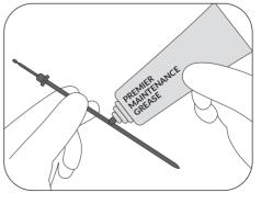
6 Lubricate the fluid needle with a small amount of maintenance grease.
