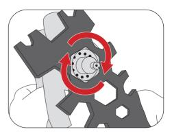
**2** Tighten it further clockwise with the universal spanner.
